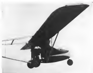
IN THE AIR The plane has a top speed of about 63 mph, lands at 25 mph. Gross weight is approximately 400 lb. It takes about a half hour to convert the plane for road travel.
